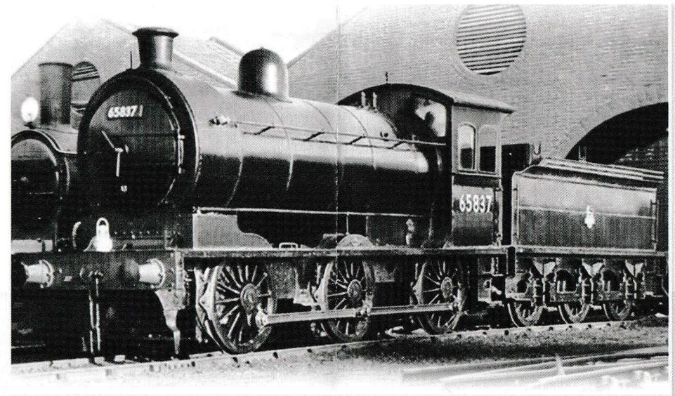
Designed by Wilson Worsdell, the NER P3 class would later be reclassified under the LNER as J27. The J27 was a modification of the earlier NER P2 (LNER J26), the biggest changes were in the depth of the firebox and shallower sloping grate. 115 engines in total were built and over their working careers received many modifications.
